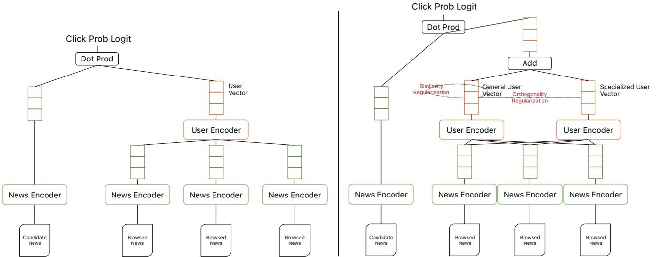
Figure 1: The comparison of the model structures of NRMS model [6] and our proposed model.
